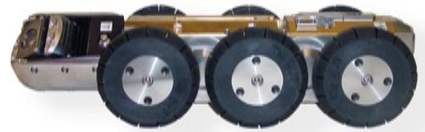
Compact Pipe Ranger in the 8" Configuration
