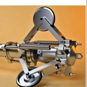
Rehabilitating old pipelines is increasingly the method of choice. However, data on the old pipeline is often inaccurate or non-existent. CUES Mapping Services has designed the Articulated AMP<sup>TM</sup> specifically to obtain digital 3D positional data for old utility pipelines.
